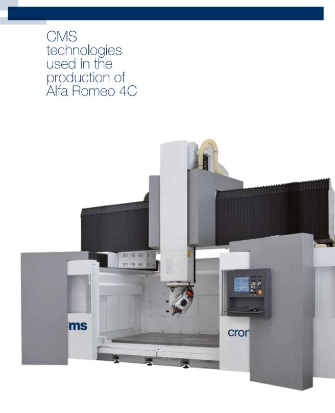
High-speed 5-axis machining centre, especially designed for the high speed machining of aluminium, light alloys and composite materials. It is provided with linear double-drive axes and rotary direct-drive axes. It ensures top-ranking speed and accelerations, along with highlevel accuracy and repeatability. Especially appreciated in the automotive industry, also owing to the superior rigidity and extensive machinable volume.
