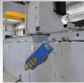
LASER SCRIBING OF MASKANT FOR CHEMICAL MILLING
