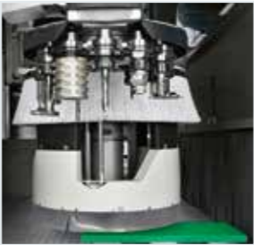
Maximum cleaning of the machine and the working environment due to the double coaxial dust extraction hood that allows the suction of shavings and sawdust in any condition of use.
