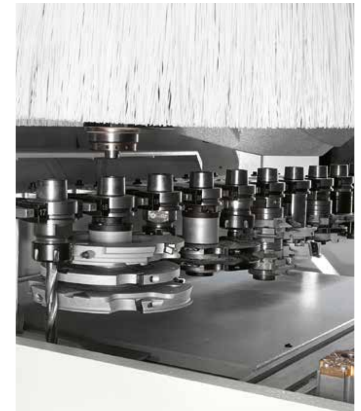
TR 12 12 positions Maximum efficiency with the side tool store positioned on the right side of the worktable.
