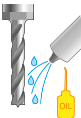
Air blower with microlubrication Air and oil-mist blower suitable for lubricating and cooling the tool in case of non-ferrous metal machining.
