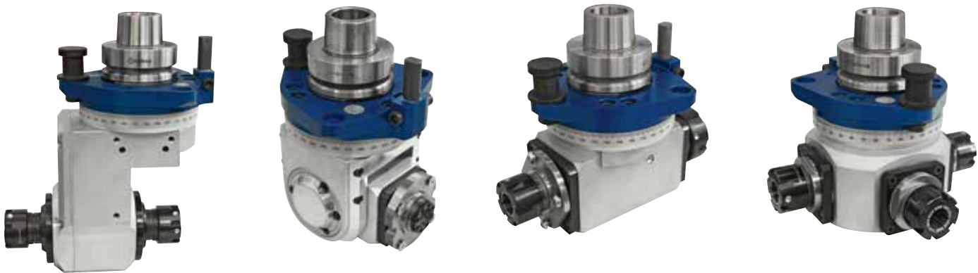
WIDE SELECTION OF CUSTOMIZATION OPTIONS TO COVER ALL NEEDS IN THE PROCESSING OF SHEETS, THERMOFORMED PARTS AND TECHNICAL ARTICLES MADE OF PLASTIC MATERIALS With angular heads having 1, 2 and 4 outlets with HSK taper couplings for angled routing, drilling and blade grooving, with plays elimination system or fixed mechanical couplings.
