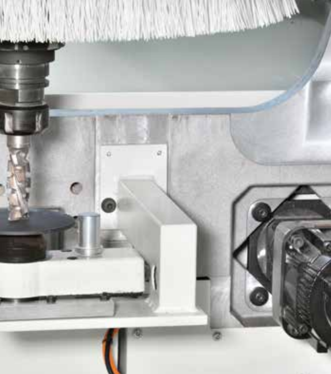
TOOL LENGTH DETECTION DEVICE Positioned on the machine base side, it allows to automatically detect the length of the tool.
