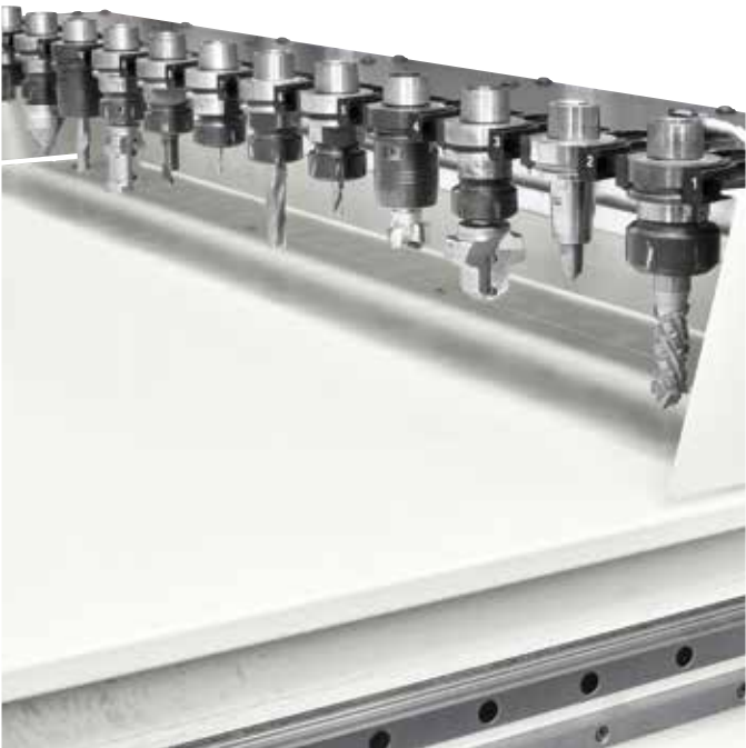
TRB side tool changer with up to 19 positions.
