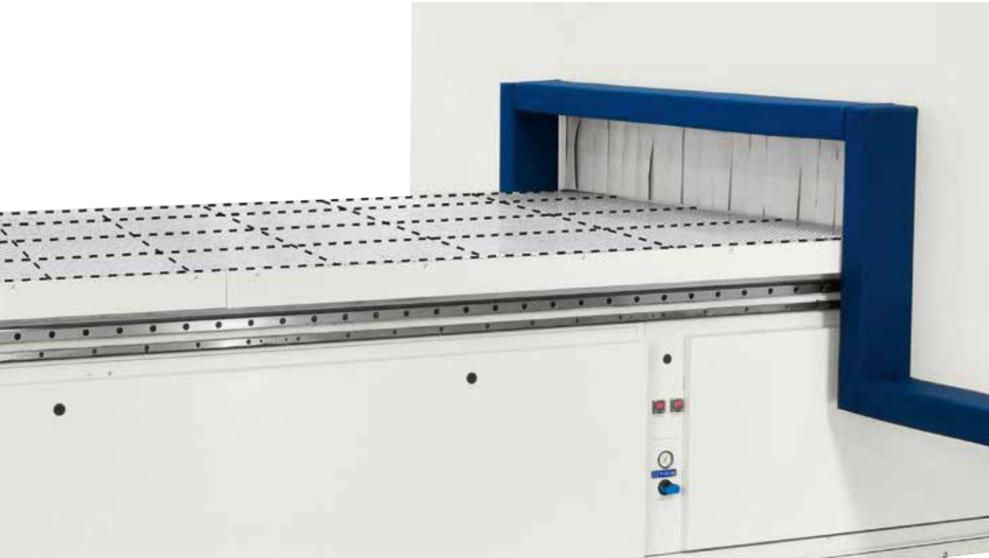
Maximum workpieces locking only where needed: starting at 2 increasing up to 30 vacuum zones according to the table size.
