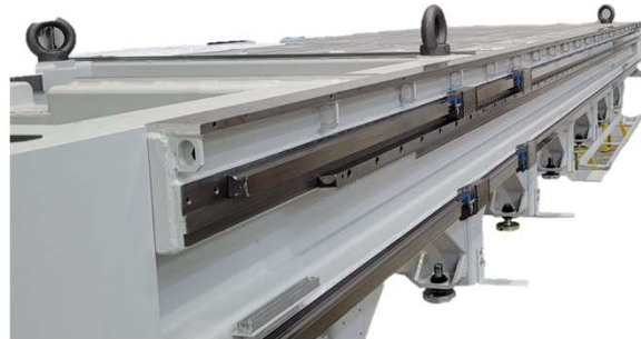
DOUBLE GUIDE for X Stroke size 35 mm
