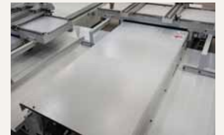
Vasche aspiranti Waste extraction tanks
