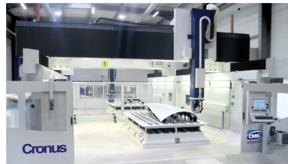
CMS Cronus machining an aircraft part
