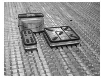
A wide selection of MPS and MODULSET suction cups to clamp workpieces to the worktable, depending on the machining to be
