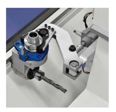
Single-position "Pick-up" magazine with pneumatic positioning anchored to the moving beam.
