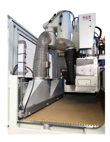
**Zero dust** and maximum plastic chip removal with the top suction system for cleaning the worktable.
