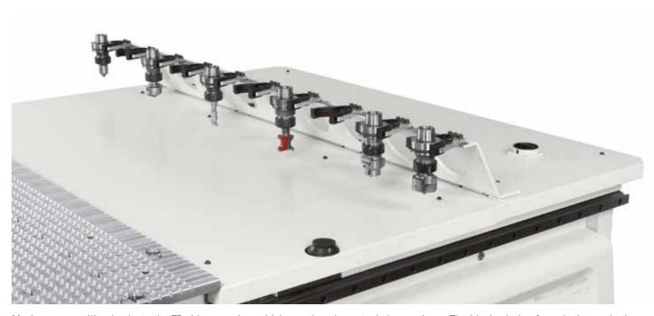
Maximum versatility thanks to the **TR** side magazine, which greatly reduces tool change times. The ideal solution for reducing cycle times, particularly when trimming flat or thermoformed plastic sheets.
